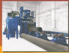
The collection and recovery system of the abrasives ensures circulation within a close cycle and efficient separation of dust.
